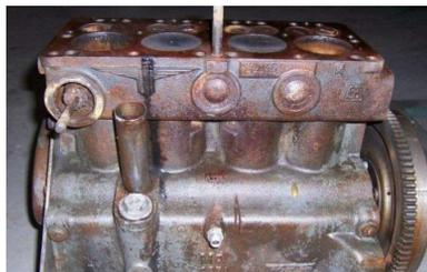
The next step is to change the damaged-, and to refurbish the worn parts of the engine. At this point, MBS profits from the product know-how of the employees. They are able to analyze the engines and to find the right parameters for the milling and drilling machines, especially for older engines, where no data sheets exists. After reassembly, MBS uses a test bench to check the performance parameters. Finally, the engine is painted and ready for delivery.
