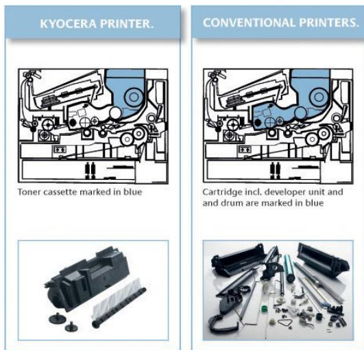
Fig. 5b KYOCERA's innovative print design demonstrating material efficiency in comparison with a conventional design
